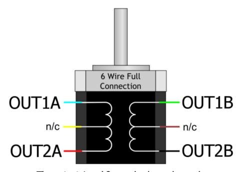
The output 1 and 2 can also be exchanged, the important thing is that output A feeds one coil and B the other.
