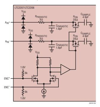
Figure 2. Equivalent Input Circuit
