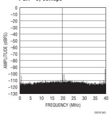
LTC2206: 64K Point FFT,  $f_{\text{IN}} = 170.2 \text{MHz}, -1 \text{dBFS},$ PGA = 1, 80Msps
