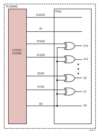
Figure 14. Descrambling a Scrambled Digital Output
