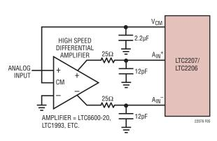
Figure 5. DC Coupled Input with Differential Amplifier
