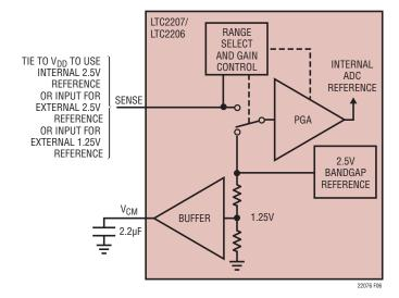
Figure 6. Reference Circuit
