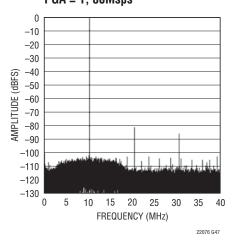
LTC2206: 64K Point 2-Tone FFT,  $f_{\text{IN}}$  = 69.2MHz and 76.5MHz, -15dBFS, PGA = 0, 80Msps
