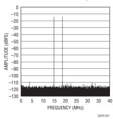
LTC2206: 64K Point FFT,  $f_{\text{IN}}$  = 25.1MHz, -1dBFS, PGA = 0, 80Msps
