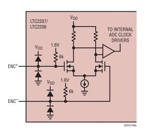
Figure 8a. Equivalent Encode Input Circuit
