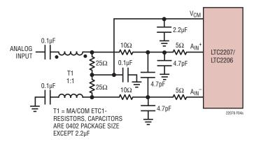
Figure 4a. Using a Transmission Line Balun Transformer.
