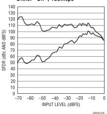
LTC2207: SFDR vs Input Level, f<sub>IN</sub> = 140MHz, PGA = 1, Dither "On", 105Msps
