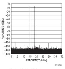
LTC2206: 64K Point 2-Tone FFT, f<sub>IN</sub> = 14.8MHz and 18.6MHz, -15dBFS, PGA = 0, 80Msps
